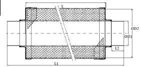
The **TSD50** fulfills all the requirements and are classified as specified within EN 13180: Ventilation for buildings – Ductwork - Dimensions and mechanical requirements for flexible ducts.
