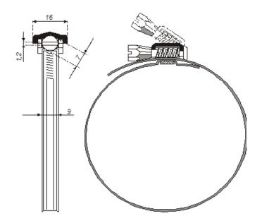
Important notice: although the product is made from Stainless steel AISI 430; due to local circumstances such as air pollution, rain, industry, traffic, climate such as sea-area, used building materials such as for the wall, temperature influences and possible chemical reactions caused by previous mentioned the material of this product is not free from possible corrosion.
