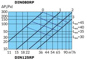
L = Sound power level in the duct dB(A).  $\Delta$ Pt(Pa)= Total pressure loss
