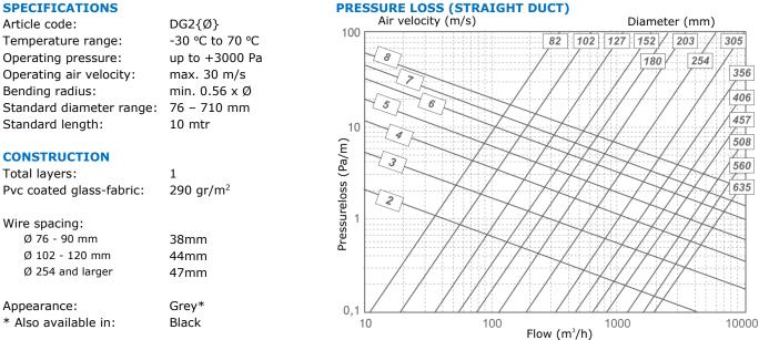
The **GREYDEC** fulfills all the requirements and are classified as specified within EN 13180: Ventilation for buildings – Ductwork - Dimensions and mechanical requirements for flexible ducts.
