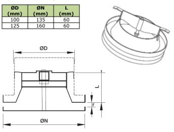
The valve is closed when the inner disc of the valve actuating element coincides with the zero-plane, Fig. Actuating valve element has only positive travel; it is totally opened when actuating valve element is moved 25 mm from the zero plane. For one turn of the valve actuating element it is longitudinally displaced for 1 mm. The graphic shows the dependence of flow rate, noise intensity and total pressure drop across the valve type **DVIR100 and DVIR125**.
